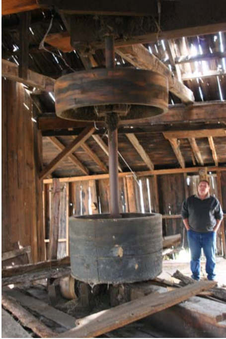
Line Shaft pulleys powered by Loeffel Water Turbine
